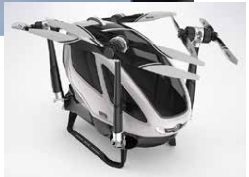
The EHang 184, was named for 'one' passenger, 'eight' propellers, and 'four' arms. When not in use, it can be folded up .
